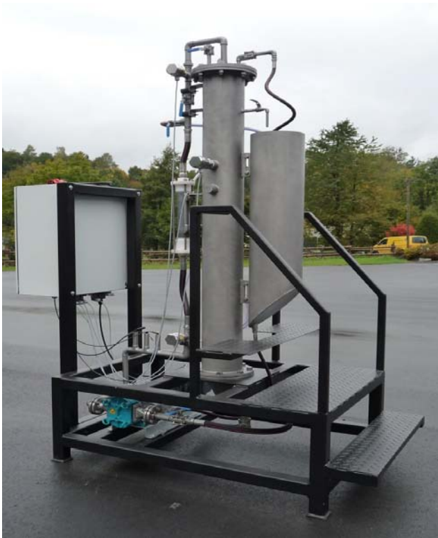
Figure 6.0 Leachox Pilot Plant
